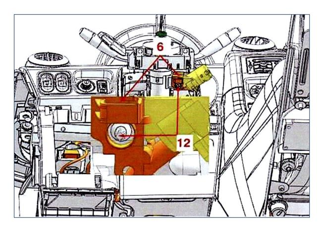
Put ignition key in position + APC If required: cut bridge 6 to make next operations
