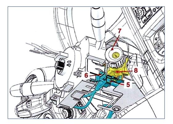
Unlock 5 from connection 6 Remove antenna transponder 7 with wiring Remove wiring 8
