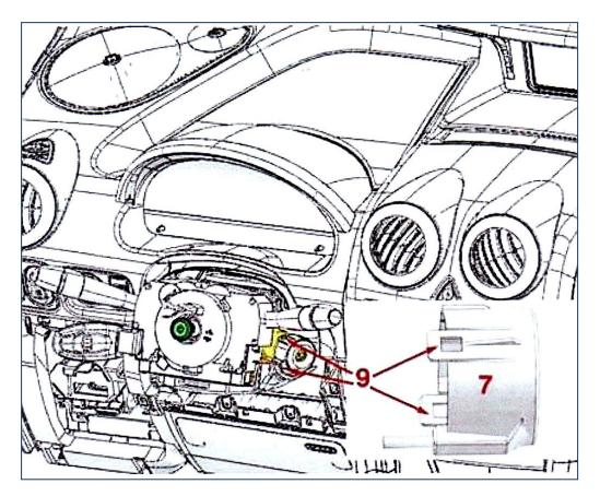
Use a small flat screw driver to unlock the locks 9
